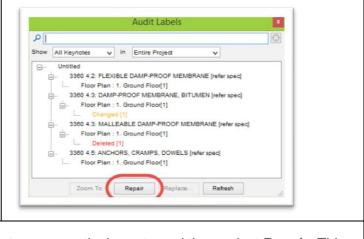
You can then select either the entire project or one particular note and then select **Repair**. This will update the Label in your ArchiCAD project with the new database entry, or it will remove it if the entry has been removed.
